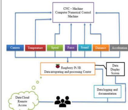
Figure 2: data and acquisition system architecture
